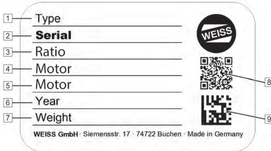
Figure 1: Example of nameplate
