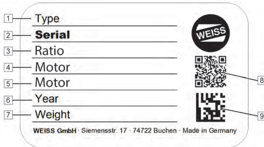
Figure 1: Example of nameplate
