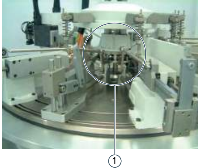
Fig. 15: Cleaning/Lubricating the guides of the central drive
